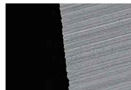
5000x zoom of an unmachined cutting edge
