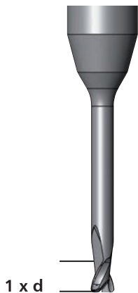
Series 570 Medium finishing and roughing flute
